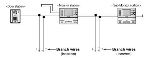
When you experience a problem with the audio or video on a sub monitor station connected to a monitor station, please terminate unused pairs of wires to prevent noise from being introduced into the monitor station.
